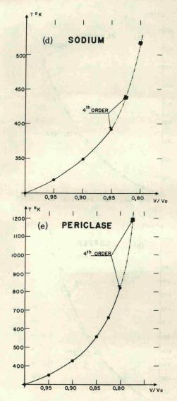
FIG. 2. Comparison of the calculated temperature (fourth-order) curves in the range of agreement of the Hugoniot and  $H_4$  curves with the data determined by Rice, McQueen, and Walsh (Ref. 6) and by McQueen and Marsh (Ref. 9) for (a) aluminum, (b) copper, (c) silver, (d) sodium, and (e) periclase.
