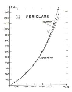
FIG. 1. Comparison of the calculated fourth-order curves  $(H_4)$  with the experimental Hugoniot curves for (a) aluminum, (b) copper, (c) silver, (d) sodium, and (e) periclase. The isotherms calculated from Eq. (9) are also shown for  $T=300\,{\rm ^\circ K}$ .
